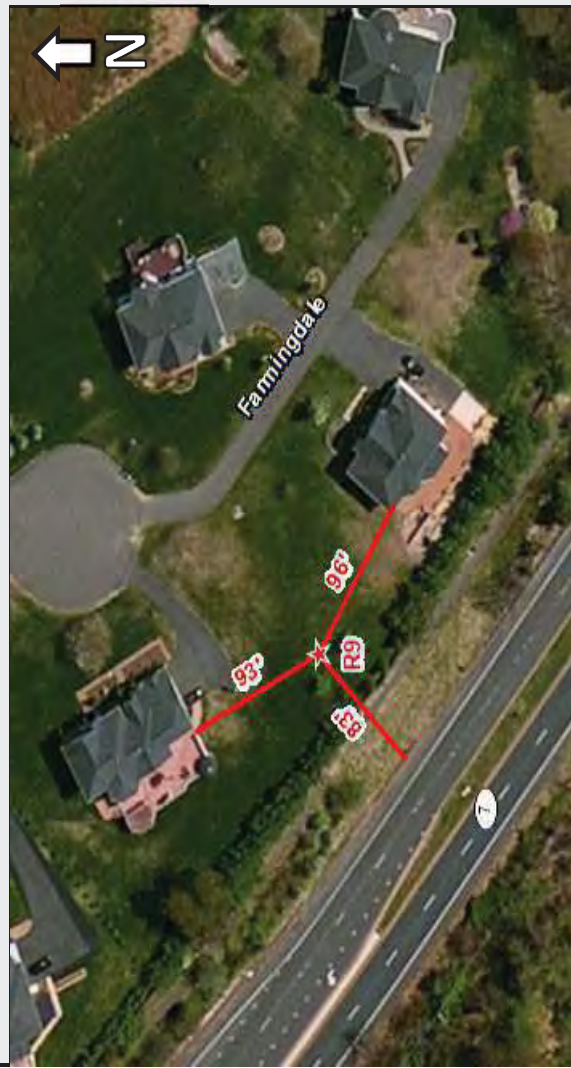
*Distances in the photo above are from noise meter to nearest structure and from noise meter to edge of pavement of the closest travel lane measured in feet.
