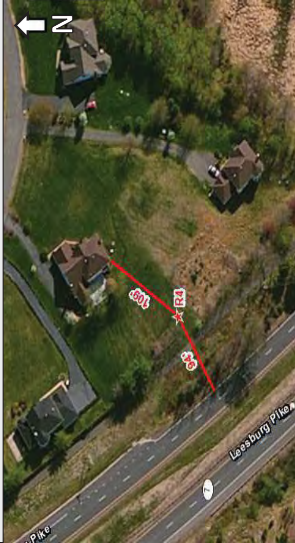
*Distances in the photo above are from noise meter to nearest structure and from noise meter to edge of pavement of the closest travel lane measured in feet.
